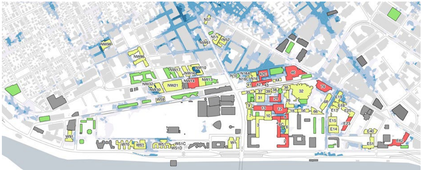
FIGURE 7 RISK TO MIT CAMPUS BUILDINGS FROM A 100-YEAR STORM UNDER CURRENT CONDITIONS
